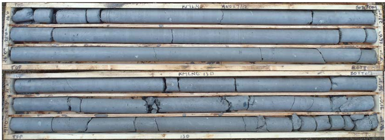
Fig. 3B Core Box Photographs showing good quality cores recovered at approximately 1.5 m (5.0 ft) runs
