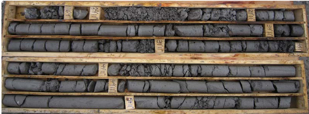
Fig. 3A Core Box Photographs showing poor quality cores recovered at approximately 1.5 m (5.0 ft) runs
